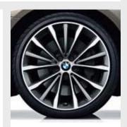
19" light alloy \W-spoke style 663 I wheels bi-colour, front 8J x 19 with 245/40 R19 tyres and rear 9J x 19 with 275/35 R19 tyres.
