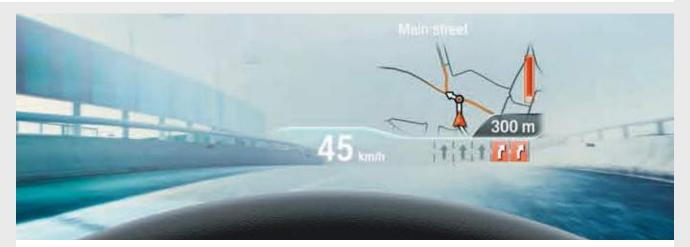
BMW Head-Up Display offers a full-colour projection of driving relevant and situational information onto the windscreen with improved resolution of 800 x 400 pixels.
