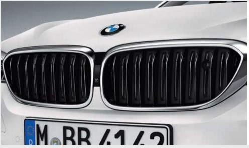
The Active Air Stream Kidney Grille knows when the engine, brakes and other components need air and automatically opens the air vents. If no further air intake is required, it closes them again. This improves aerodynamics and fuel consumption falls.
