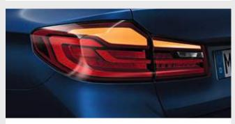
The **LED Rear Lights** are split into two parts, with LED technology featured in the tail lights, brake lights, turn indicators and reversing lights.
