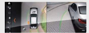
Parking Assistant with Surround View Camera makes parking and manoeuvring the vehicle easier. The Parking Assistant with linear guidance parks the vehicle automatically, parallel or perpendicular to the street. If the driver parks manually without the help of the Parking Assistant, Active Park Distance Control (PDC) offers additional protection against damage with the Lateral parking aid.
