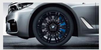
19" M light alloy Double-spoke style 664 M wheels, Black, front  $8J \times 19$  with 245/40 R19 tyres and rear  $9J \times 19$  with 275/35 R19 tyres.
